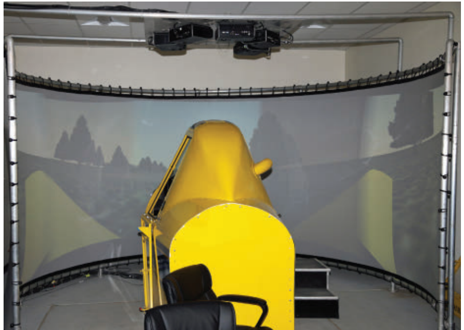
HIGH-DEF UPGRADE The UNL Pesticide Application Technology Laboratory recently installed new high-definition projectors to enhance the scenes shown on the 235-degree screen of its AT-502 simulator.
